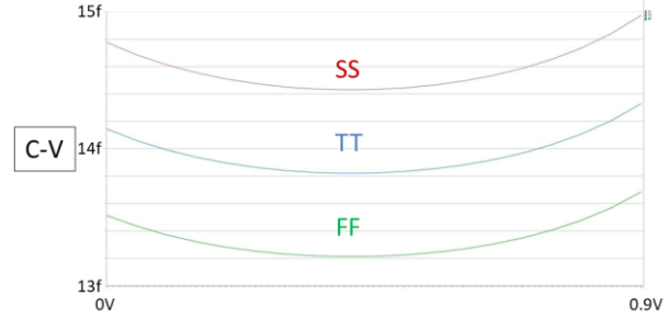
Figure 18: Simulation of the parasitic capacitance of the 15fF version on 7nm, across applied IO voltage and for 3 corners.
